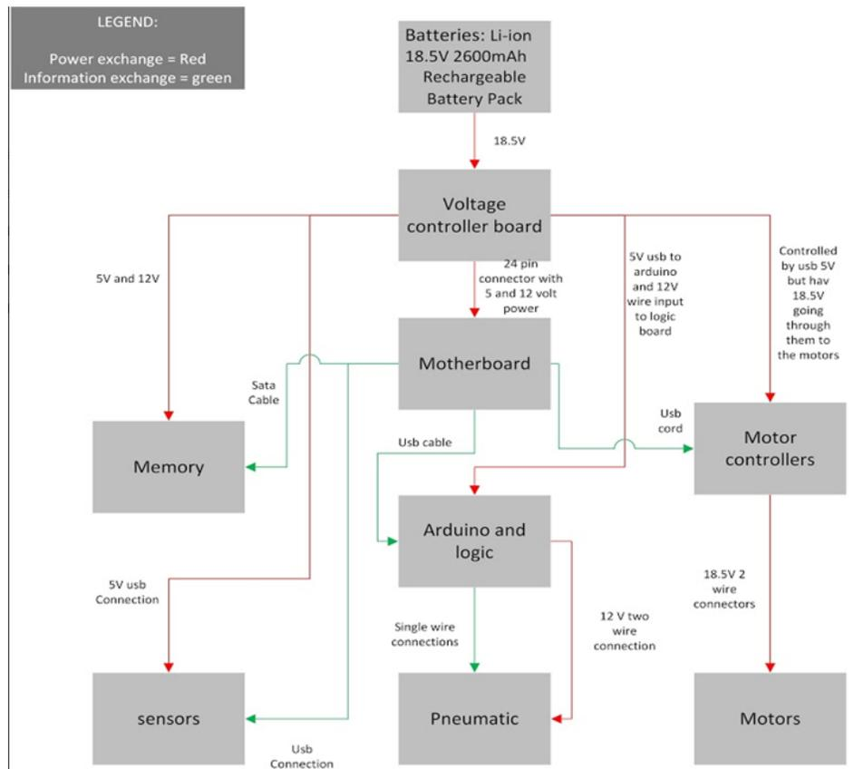
Figure 6 – Electrical System Block Diagram
