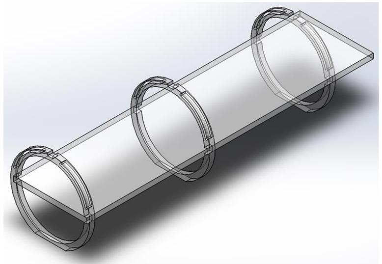
**Figure 5** – Solidworks model of electronics rack. Rectangular key ways are shown at top.
