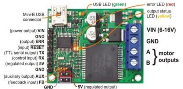
Figure 8 – Top view of the motor controller with pin information
