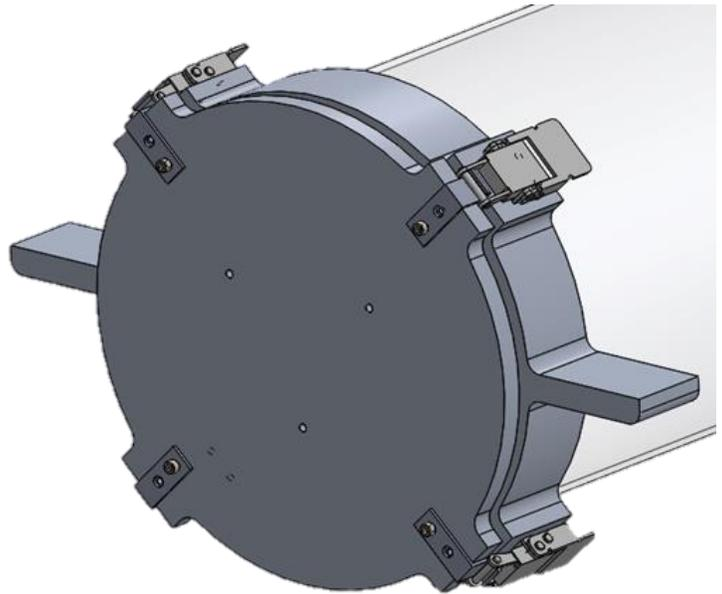
Figure 3 – Solidworks model of the rear endcap with latch mechanisms
