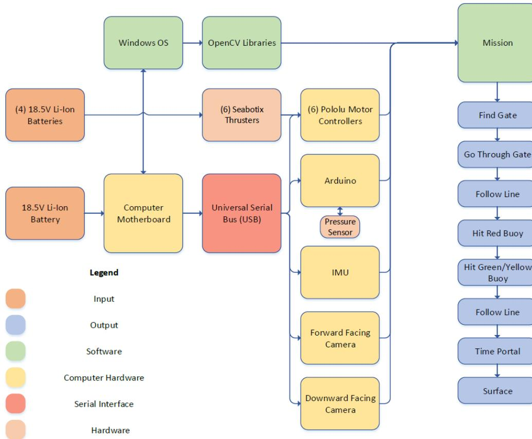
Figure 11 – Software Block Diagram
