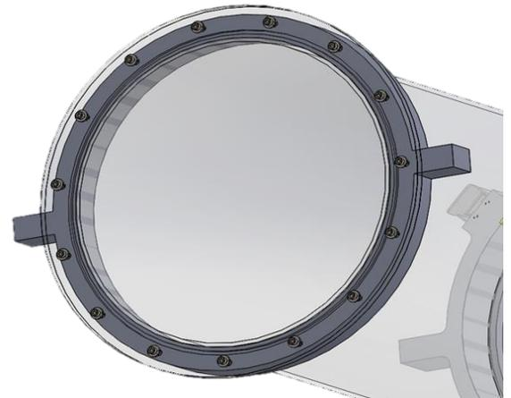
**Figure 4** – Solidworks model of the clear front end cap
