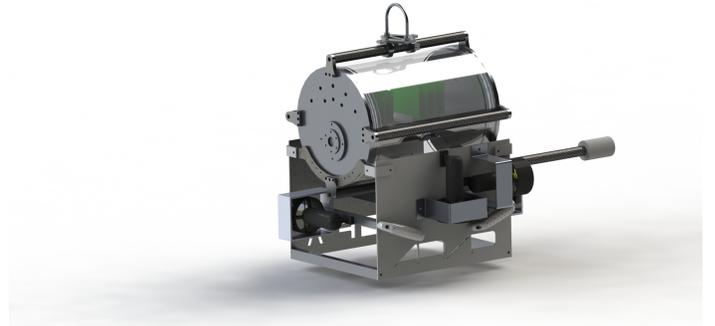
Fig. 1. Solid rendering of AquaUrsa's complete hull.
