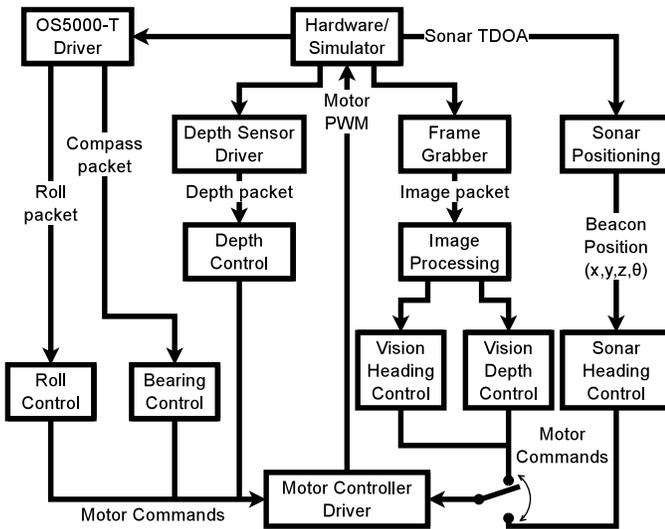
Fig. 2. Overview of software components and their interaction.
