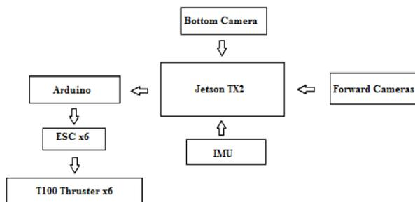
Figure 2. Block Diagram of the Connections for the Jetson Tx2
