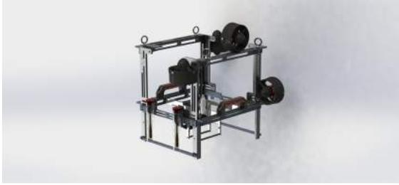
Fig. 15: A Solidworks rendering of Loki's frame
