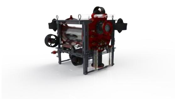
Fig. 14: A SolidWorks rendering of CUAUV's 2016 secondary vehicle, Loki
