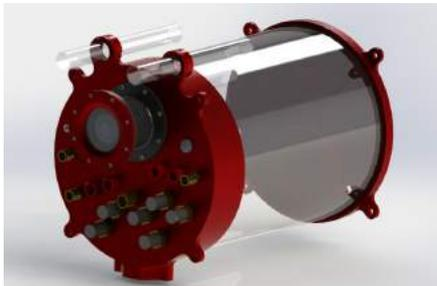
Fig. 16: A SolidWorks rendering of Loki's UHPV
