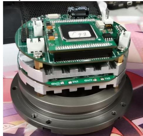
Figure 5 : USBL system electronic board
