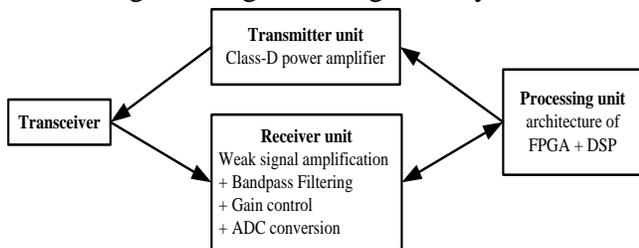
Figure 8: Hardware scheme of underwater acoustic communication system
