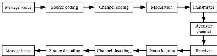
Figure 7: Physical system block diagram of underwater acoustic communication
