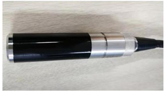
Figure 9: Physical diagram of transceiver transducer
