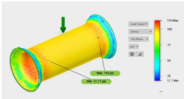
Fig. 3 Stress Analysis for the Hull
