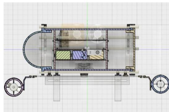
Fig. 17 Autodesk Fusion Rendering of CM and CB Coordinate Results
