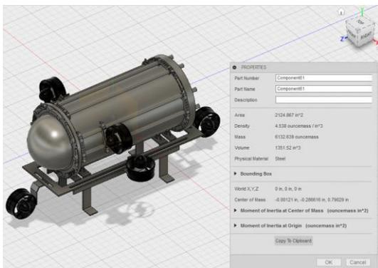
Fig. 16 Autodesk Fusion Rendering of Center of Buoyancy Calculations
