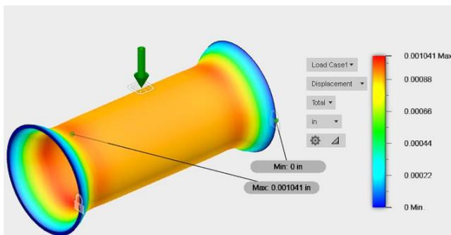
Figure 4. Displacement Analysis for Hull
