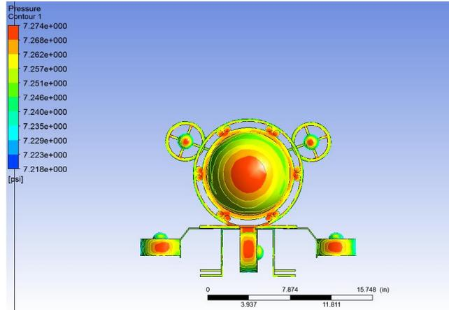
Fig. 12 ANSYS rendering of a Pressure Contour Analysis (Front View)
