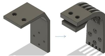
Fig. 21 Autodesk Fusion Rendering comparison of old to new updated L-brackets for Thrusters
