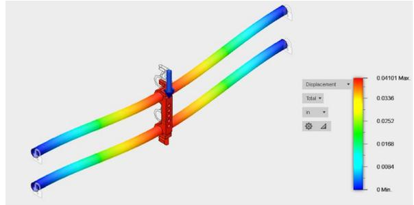
Fig. 15 Displacement Analysis of Camera Rods with Rod Clamp
