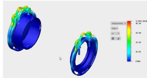
Fig. 9. Displacement Analysis of the Front and Back Endcaps
