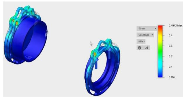
Fig. 8 Stress Analysis of the Front and Back Endcaps
