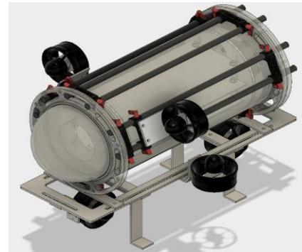
Fig. 2 Autodesk Fusion CAD rendering of the original *PV Inspire*
