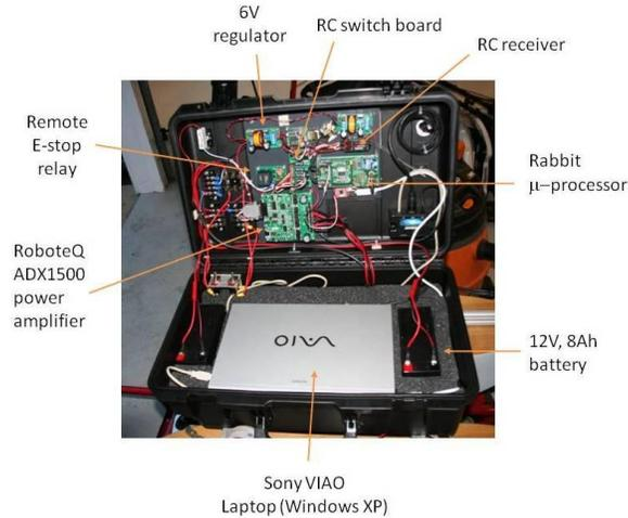
**Figure 6: The electrical layout**
