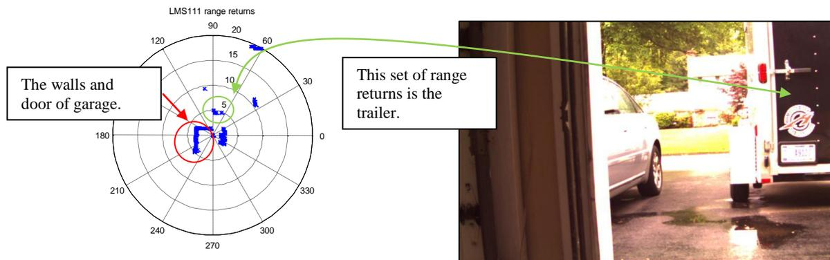
**Figure 5: (a) Sample laser return and (b) the corresponding acquired image**
