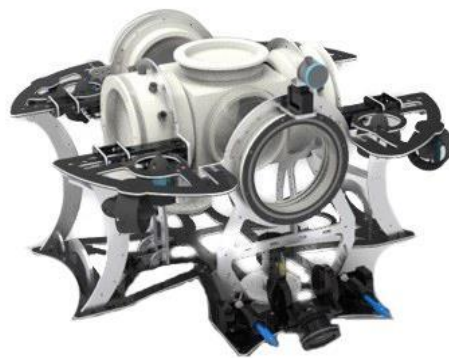
Fig. 1: AUV Final design featuring a rigid "sandwich" frame and hull inlets
