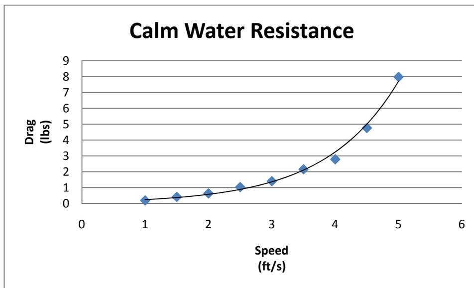
Figure 1 Calm water Resistance data (Davidson Laboratory high speed towing tank)
