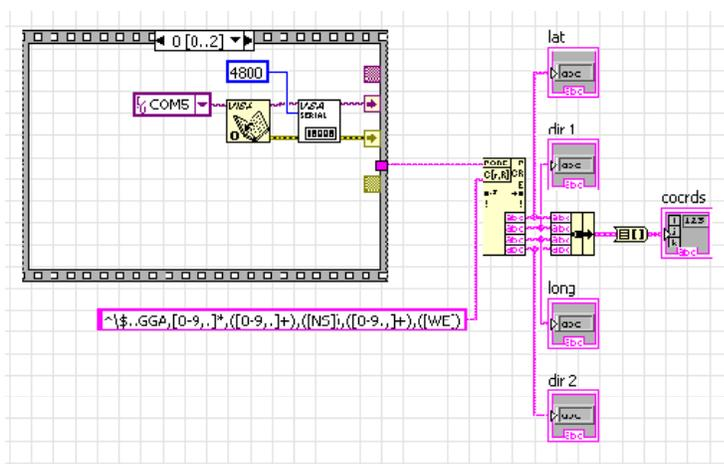
Figure 9: An example of LabView graphical programming language to retrieve coordinates from the GPS device.
