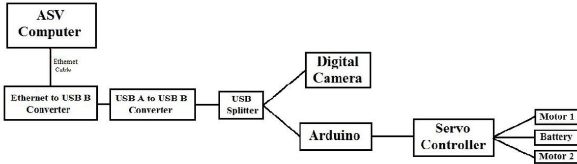
Figure 6 Electrical diagram connecting the rover to the main computer
