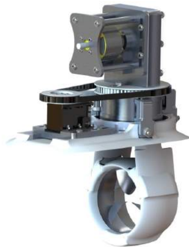
Figure 7. Assembly of PropaGator 2's propulsion system
