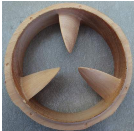
Figure 8. Hubless propeller designed and manufactured for this project
