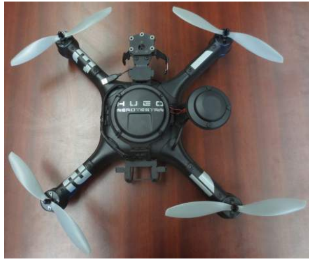
Figure 9. HUGO, a waterproof quadcopter used by PropaGator 2
