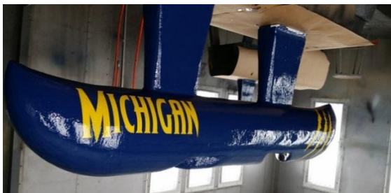
Figure 8: Hulls after decals and final epoxy coat added.
