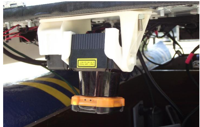
Figure 10: A photo of the 3D printed rocking Lidar mount.
